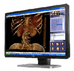
Vision Tools 3Dview is a three dimension reconstruction software designed to make 3D volume in colors for ultrasound, CT and MRI machines simultaneously, 3DView can make MRP/3D volume, adjust the view mode of the 3D volume, navigate through the volume, adjust the volume opacity to change the window and level of the display thus you can see Bone and Soft tissue for CT, ..
